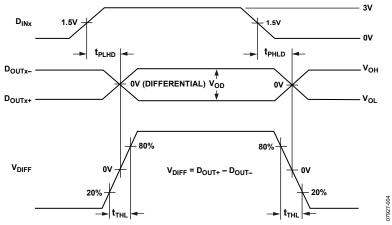
Figure 4. Driver Propagation Delay and Transition Time Waveforms
