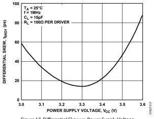
Figure 17. Differential Skew vs. Power Supply Voltage
