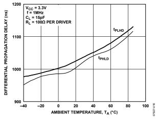
Figure 16. Differential Propagation Delay vs. Ambient Temperature
