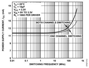
Figure 12. Power Supply Current vs. Switching Frequency
