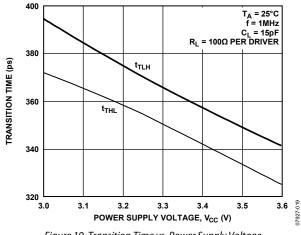
Figure 19. Transition Time vs. Power Supply Voltage
