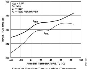
Figure 20. Transition Time vs. Ambient Temperature
