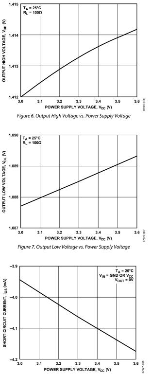
Figure 8. Output Short-Circuit Current vs. Power Supply Voltage
