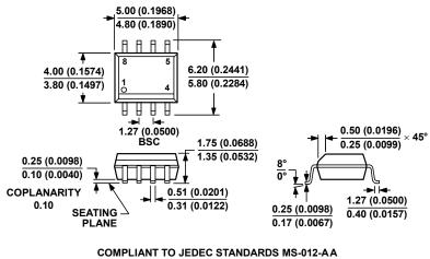
COMPLIANT TO JEDEC STANDARDS MS-012-AA CONTROLLING DIMENSIONS ARE IN MILLIMETERS; INCH DIMENSIONS (IN PARENTHESES) ARE ROUNDED-OFF MILLIMETER EQUIVALENTS FOR REFERENCE ONLY AND ARE NOT APPROPRIATE FOR USE IN DESIGN.
