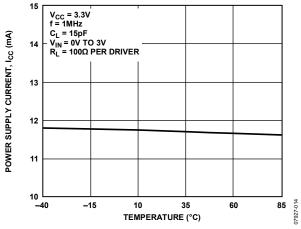
Figure 14. Power Supply Current vs. Ambient Temperature
