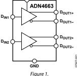
twisted-pair cable. The transmitted signal develops a differential voltage of typically  $\pm 355$  mV across a termination resistor at the receiving end, and this is converted back to a TTL/CMOS logic level by a line receiver.
