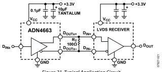
Figure 21. Typical Application Circuit
