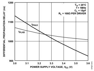
Figure 15. Differential Propagation Delay vs. Power Supply Voltage
