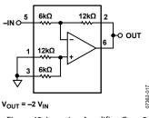
Figure 43. Inverting Amplifier, G = -2
