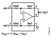
*Figure 40. Difference Amplifier,*  $G = \frac{1}{2}$
