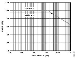
Figure 15. Common-Mode Rejection Ratio vs. Frequency, Referred to Input
