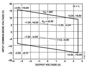
Figure 9. Input Common-Mode Voltage vs. Output Voltage, Gain =  $\frac{1}{2}$ ,  $\pm 5$  V and  $\pm 2.5$  V Supplies
