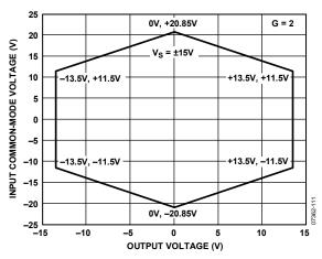
Figure 10. Input Common-Mode Voltage vs. Output Voltage, Gain = 2,  $\pm 15$  V Supplies
