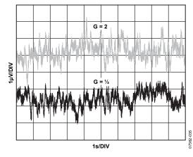
Figure 31. 0.1 Hz to 10 Hz Voltage Noise, RTO
