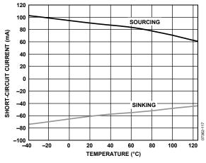
Figure 16. Short-Circuit Current vs. Temperature
