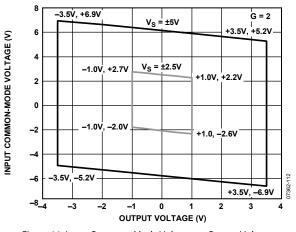
Figure 11. Input Common-Mode Voltage vs. Output Voltage, Gain = 2,  $\pm$ 5 V and  $\pm$ 2.5 V Supplies
