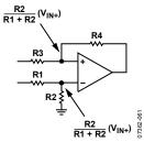
Figure 39. Voltage Division in the Difference Amplifier Configuration
