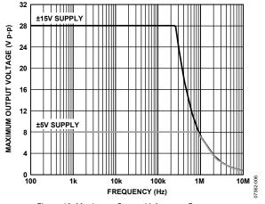
Figure 13. Maximum Output Voltage vs. Frequency
