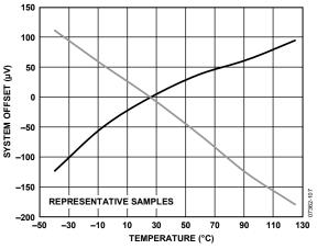
Figure 6. System Offset vs. Temperature, Normalized at 25°C, Referred to Output, Gain = ½
