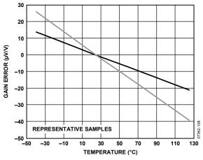
Figure 7. Gain Error vs. Temperature, Normalized at 25°C, Gain = 1/2
