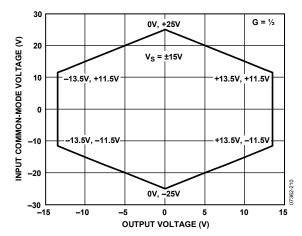
Figure 8. Input Common-Mode Voltage vs. Output Voltage, Gain =  $\frac{1}{2}$ ,  $\pm 15$  V Supplies
