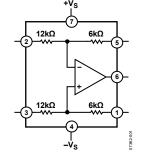
Figure 38. Functional Block Diagram
