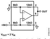
Figure 45. Noninverting Amplifier, G = 2
