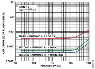
Figure 37. Harmonic Distortion Products vs. Frequency, G = 2
