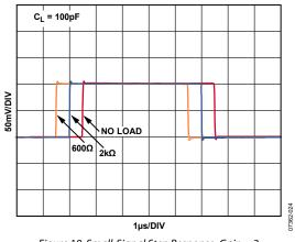
Figure 19. Small-Signal Step Response, Gain = 2
