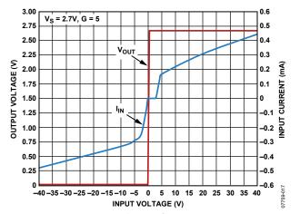
Figure 17. Input Overvoltage Performance, G = 5,  $V_s = 2.7 \text{ V}$
