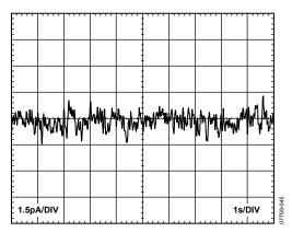
Figure 45. 0.1 Hz to 10 Hz Current Noise
