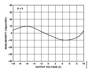
Figure 38. Gain Nonlinearity, G = 5,  $R_L \ge 2 k\Omega$
