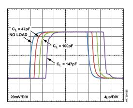
Figure 55. Small-Signal Pulse Response with Various Capacitive Loads,  $G=5, R_L=Infinity$
