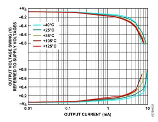
Figure 37. Output Voltage Swing vs. Output Current
