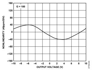
Figure 40. Gain Nonlinearity, G = 100,  $R_L \ge 2 \text{ k}\Omega$
