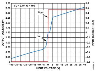
Figure 19. Input Overvoltage Performance, G = 100,  $V_s = 2.7 \text{ V}$
