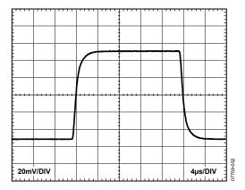
Figure 52. Small-Signal Pulse Response, G = 10,  $R_L = 10$  k $\Omega$ ,  $C_L = 100$  pF
