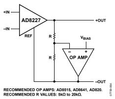
Figure 64. Differential Output Using an Op Amp
