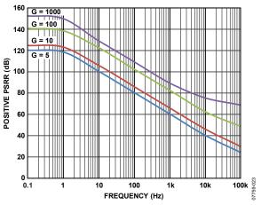
Figure 23. Positive PSRR vs. Frequency, RTI
