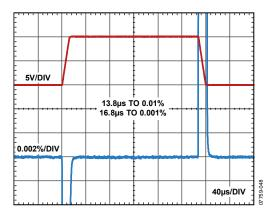
Figure 48. Large-Signal Pulse Response and Settling Time, G = 10, 10 V Step,  $V_S = \pm 15 \text{ V}$
