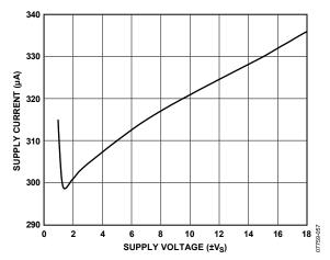
Figure 57. Supply Current vs. Supply Voltage
