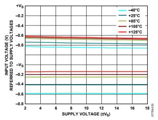
Figure 33. Input Voltage Limit vs. Supply Voltage
