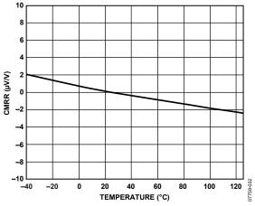
Figure 32. CMRR vs. Temperature, G = 5
