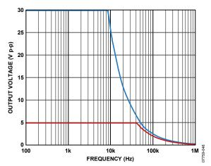
Figure 46. Large-Signal Frequency Response
