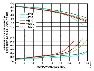
Figure 35. Output Voltage Swing vs. Supply Voltage,  $R_L = 2 k\Omega$
