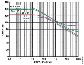
Figure 27. CMRR vs. Frequency, RTI
