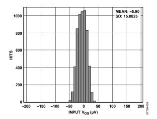
Figure 5. Typical Distribution of Input Offset Voltage
