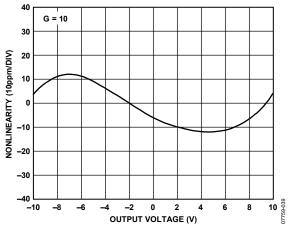
Figure 39. Gain Nonlinearity, G = 10,  $R_L \ge 2 k\Omega$
