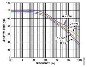
Figure 24. Negative PSRR vs. Frequency
