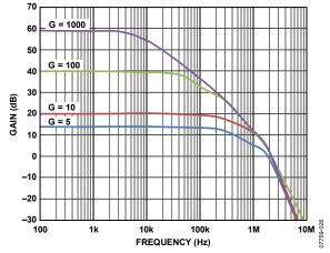
Figure 26. Gain vs. Frequency,  $V_S = 2.7 \text{ V}$
