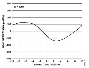
Figure 41. Gain Nonlinearity, G = 1000,  $R_L \ge 2 \text{ k}\Omega$
