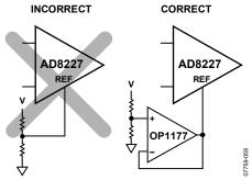
Figure 59. Driving the Reference Pin
