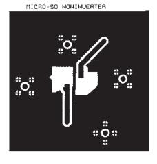
Figure 13. Universal MSOP Noninverter Bottom
