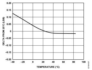
Figure 7. Change in Gain vs. Temperature
