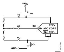
Figure 29. Differential Reference Mode (SER/ $\overline{DFR} = 0$ )
