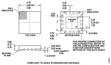
Figure 42. 16-Lead Lead Frame Chip Scale Package [LFCSP\_WQ] 4 mm × 4 mm Body, Very Very Thin Quad (CP-16-23) Dimensions shown in millimeters
