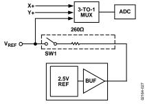
Figure 27. On-Chip Reference Circuitry
