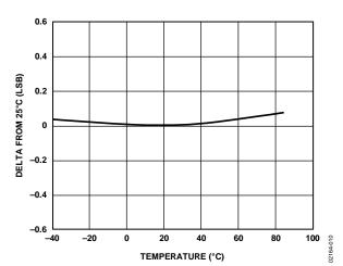
Figure 10. Change in Offset vs. Temperature
