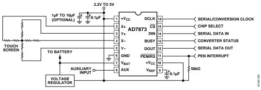
Figure 25. Typical Application Circuit
