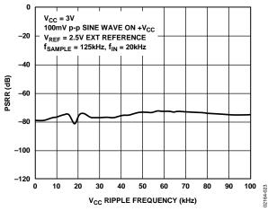
Figure 23. AC PSRR vs. Supply Ripple Frequency
