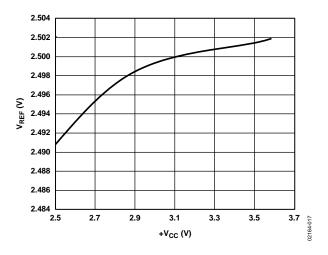
Figure 17. Internal  $V_{REF}$  vs.  $+V_{CC}$
