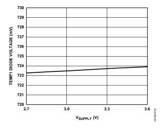
Figure 19. TEMP1 Diode Voltage vs. V<sub>SUPPLY</sub> (25°C)
