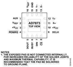
Figure 3. LFCSP Pin Configuration
