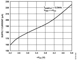
Figure 6. Supply Current vs.  $+V_{CC}$
