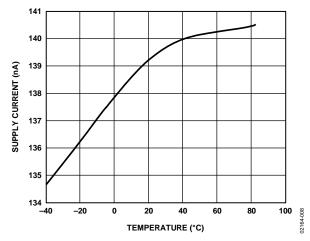
Figure 8. Power-Down Supply Current vs. Temperature
