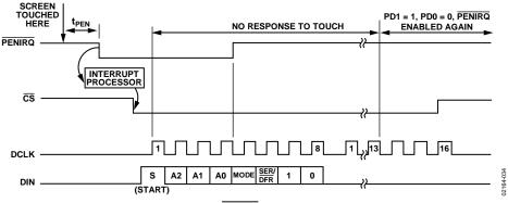
Figure 34. PENIRQ Timing Diagram
