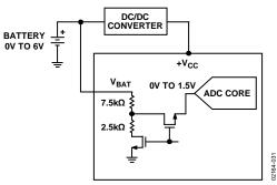
Figure 31. Block Diagram of Battery Measurement Circuit
