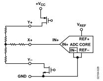
Figure 28. Single-Ended Reference Mode (SER/ $\overline{DFR} = 1$ )
