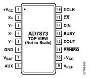
Figure 4. QSOP/TSSOP Pin Configuration
