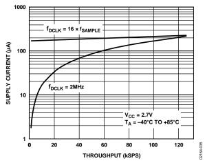
Figure 35. Supply Current vs. Throughput (μA)
