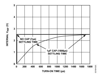
Figure 20. Internal V<sub>REF</sub> vs. Turn-on Time
