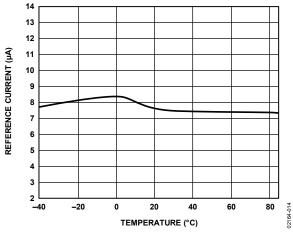
Figure 14. Reference Current vs. Temperature
