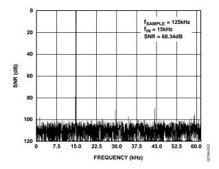
Figure 22. Auxiliary Channel Dynamic Performance (f<sub>SAMPLE</sub> = 125 kHz, f<sub>INPUT</sub> = 15 kHz)
