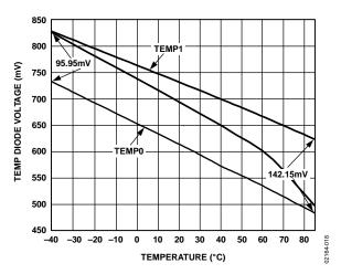
Figure 18. Temp Diode Voltage vs. Temperature (2.7 V Supply)
