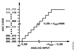
Figure 24. Transfer Characteristic
