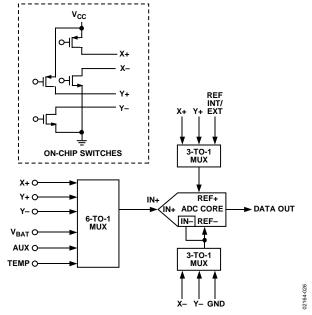
Figure 26. Equivalent Analog Input Circuit
