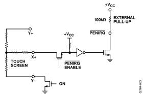
Figure 33. PENIRQ Functional Block Diagram
