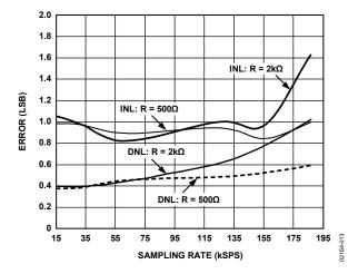
Figure 13. Linearity Error vs. Sampling Rate for Various R<sub>IN</sub>
