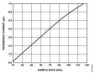
Figure 11. Reference Current vs. Sample Rate
