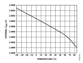
Figure 16. Internal V<sub>REF</sub> vs. Temperature
