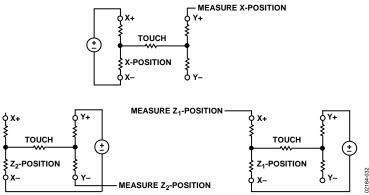
Figure 32. Pressure Measurement Block Diagram
