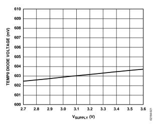
Figure 21. TEMPO Diode Voltage vs. V<sub>SUPPLY</sub> (25°C)
