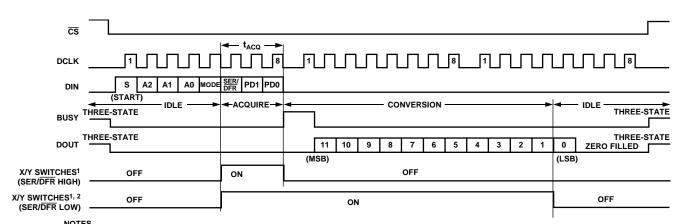
TY DRIVERS ARE ON WHEN X+ IS SELECTED INPUT CHANNEL (A2 TO A0 = 001); X DRIVERS ARE ON WHEN Y+ IS SELECTED INPUT CHANNEL (A2 TO A0 = 101).
