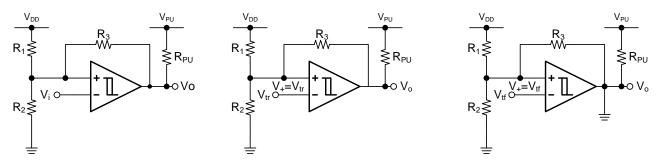
Figure 5. Inverting Configuration with Hysteresis
