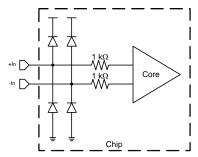
Figure 2. Equivalent Input Structure
