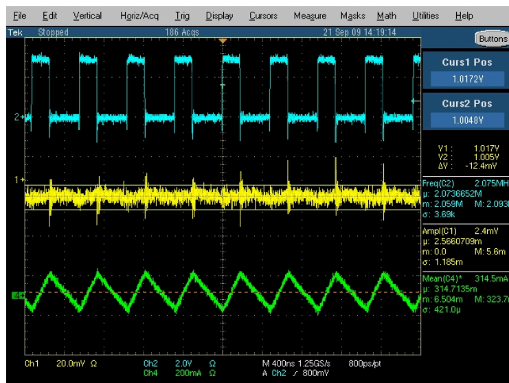
Figure 15. L=GLK2510P-2R2M, C=Ceramic 4.7 \mu F 0805 X5R TDK (Ripple 12.4mV)
