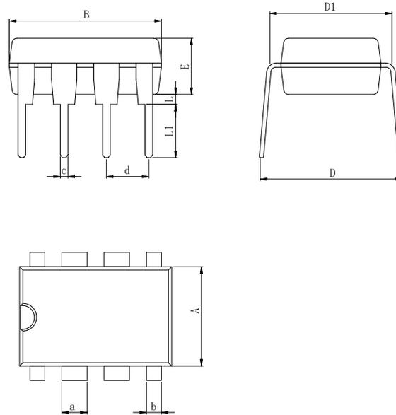
**Dimensions In Millimeters(DIP-8)**
