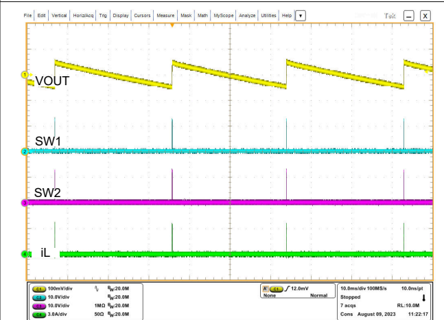
Figure 8-5. Switching Waveforms in V_{IN} = 12\text{ V} , V_{OUT} = 12\text{ V} , I_O = 0\text{ A} , PFM
