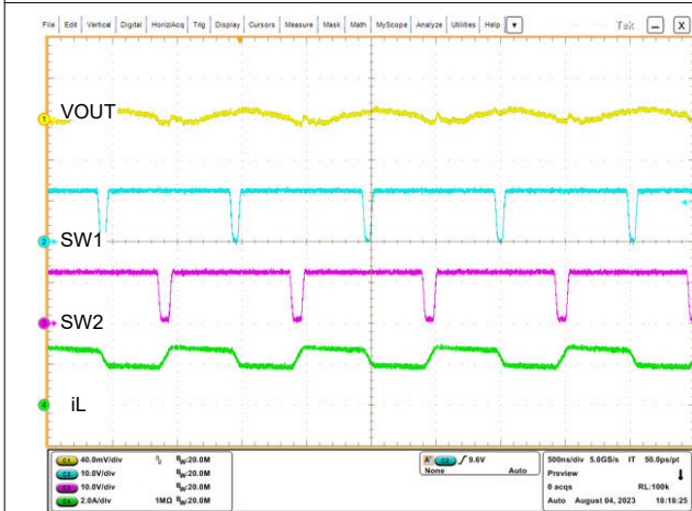
Figure 8-4. Switching Waveforms in V_{IN} = 12\text{ V} , V_{OUT} = 12\text{ V} , I_O = 2\text{ A} , FPWM
