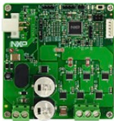
S12ZVM-EFP Electrical Fuel Pump S12ZVML128 reference design
