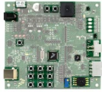
VLG-MC9S12ZVC CAN node S12ZVC192 evaluation board
