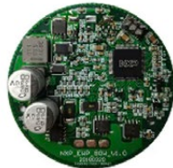
S12ZVM-EWP Electrical Water Pump S12ZVML64 reference design
