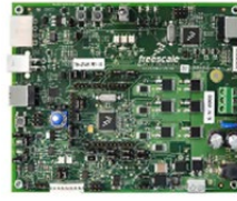
S12ZVMEVB 3-phase BLDC and PMSM S12ZVM(L/C)128 evaluation board
