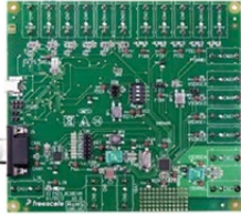
KIT9Z1J638EVM battery monitoring MM912J638 evaluation board
