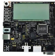
TRK-S12ZVFP64 Instrument cluster S12ZVFP64 evaluation board
