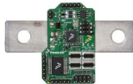
RD9Z1-638-4Li 14.4 V battery monitoring MM912J638 reference design
