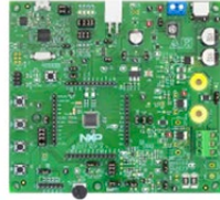
S12ZVMAEVB Unidirectional DC S12ZVMA evaluation board
