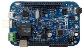
DEVKIT-S12VR64 Relay-based DC S12VR64 evaluation board
