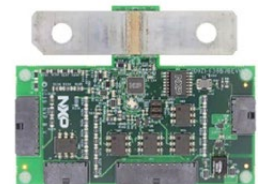
RD9Z1-638BJBEVM Battery junction box MM912J638 reference design
