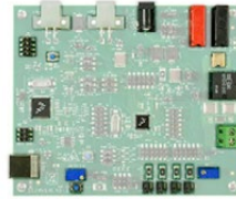
S12VR64EVB3 Relay-based DC S12VR64 evaluation board
