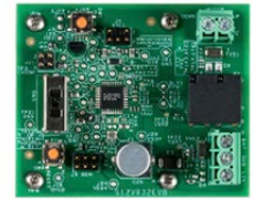
S12VR32EVB Relay-based DC S12VR32 evaluation board
