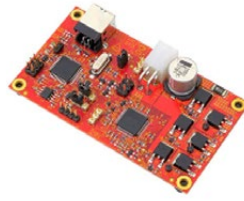
S12ZVML-MINIXXX 3-phase PMSM Motor control kit
