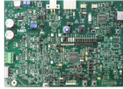
S12ZVMC256EVB 3-phase BLDC and PMSMS12ZVMC256 evaluation board
