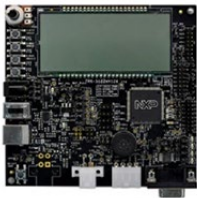
TRK-S12ZVH128 Instrument cluster S12ZVH128 evaluation board
