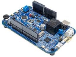
DEVKIT-S12VRP Relay-based DC S12VRP64 evaluation board
