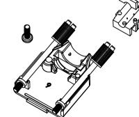
BACKSHELL MATERIAL: PLATING: JACKSCREWS: M3 HOODSCREWS: COMPRESSION INSERT: DIE-CAST ZINC ALLOY CLEAR CHROMATE FOLLOWED BY BLACK ENAMEL STEEL:ZN PLATED WITH PLASTIC KNOB BLACK STEEL:BLACK OXIDE FINISH ABS.BLACK COLOR.UL RECOGNIZED
