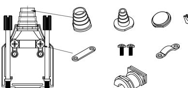
BACKSHELL: MATERIAL: PLATING: COMPRESSION INSERT: 4-40 THUMBSCREWS: HOUSING SCREWS: STRAIN RELIEF CLAMP: STRAIN RELIEF SCREWS: OPERATING TEMP: DIE CAST ZINC ALLOY NICKEL PLATED ABS-UL RECOGNIZED STEEL-Zn PLATED STEEL-Zn PLATED STEEL-NICKEL PLATED STEEL-Zn PLATED -40°C TO+120°C
