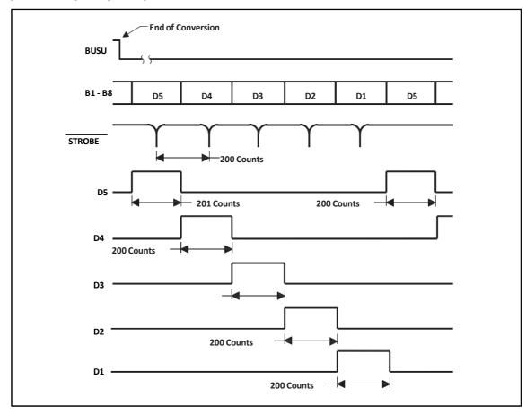
$\label{eq:decomposition} \textbf{Delay between BUSY going low and the first STROBE pulse is dependent upon the analog input.}$
