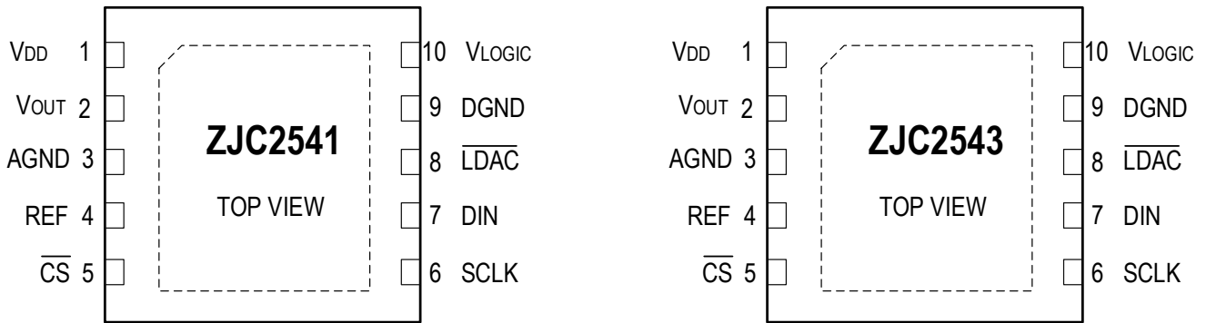
Figure 5. ZJC2541 and ZJC2543 with the same 10 - Pin DFN Pinout Diagram
