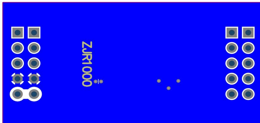
Figure 28. ZJR1000 Evaluation Board Layout (Bottom Layer)
