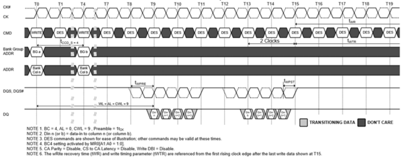
Figure 137. WRITE (BC4) Fixed to WRITE (BC4) Fixed with 1tCK Preamble in Different Bank Group
