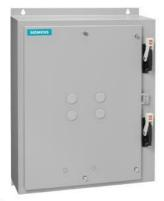
Duplex starter w/ alternator, Size 4, Three phase full voltage, Solid-state overload relay, OLR amp range 50-200A, 110V 50Hz / 120V 60Hz coil, Combination type, Two 150A circuit breakers, Enc NEMA type 4 painted steel, Water/dust tight for outdoors
