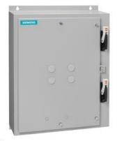
Duplex starter w/o alternator Size 3 Three phase full voltage Solid-state overload relay OLR amp range 25-100A 240VAC 50Hz / 277VAC 60Hz Coil Combination type Two 100A disconnect switches Encl NEMA type 4 painted steel Water/dust tight weather proof
