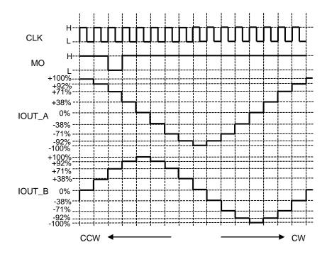
MO is a waveform of the pin output in pull-up state.
