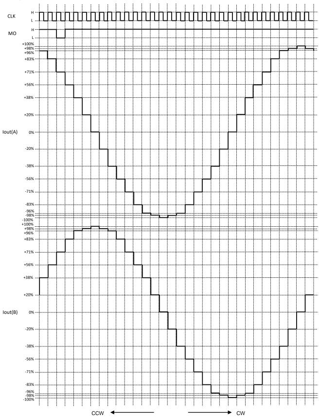
MO is a waveform of the pin output in pull-up state.
