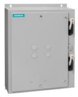
Duplex starter w/o alternator Size 1 Three phase full voltage Solid-state overload relay OLR amp range 0.75-3.4A 240VAC 50Hz / 277VAC 60Hz Coil Combination type Two 30A disconnect switches Enclosure NEMA type 4/12 Water/dust tight weather proof
