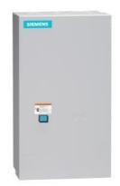
Non-reversing motor starter, Size 3 1/2, Three phase full voltage, Amb. compensate bimetal OLR, Contactor amp rating 115A, 24VDC coil, Noncombination type, Enclosure type 1, Indoor general purpose use
