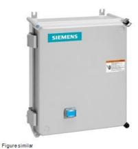
Non-reversing motor starter, Size 1, Three phase full voltage, Solid-state overload relay, OLR amp range 10-40A, 240V 50Hz / 277V 60Hz coil, Non-combination type, Enclosure type 4X fiberglass, Water/dust tight noncorrosive, Standard width enclosure
