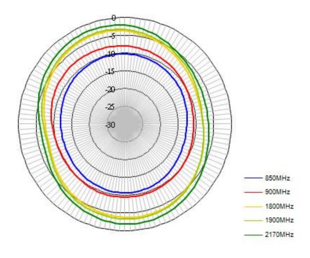
A. Radiation Pattern, Azimuth Plane (XY)
