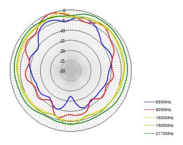
B. Radiation Pattern, Aligned at the Connector
