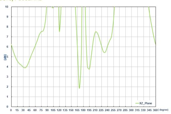
XZ Plane (phi=0  $^{\circ}\,$  , Theta= -180~180  $^{\circ}\,$  ), 0 degree face Zenith
