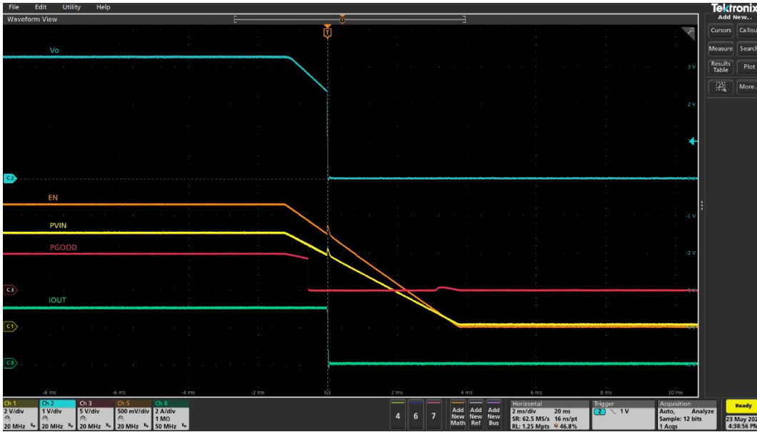
Figure 15 Shutdown with VCC UVLO at 3A load (Ch1: PV IN , Ch2: V OUT , Ch3: PG, Ch5: Enable, Ch8: I OUT )
