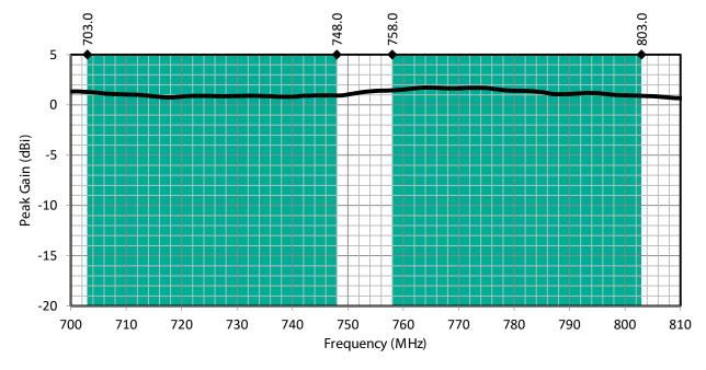
Figure 3: CW LTE Band 28 Antenna Peak Gain with Band 28 Uplink/Downlink Highlights
