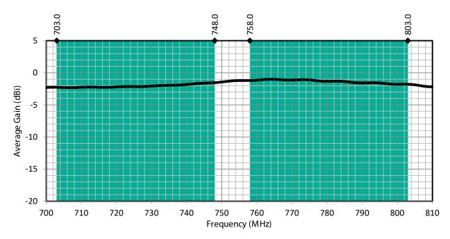
Figure 4: CW LTE Band 28 Antenna Average Gain with Band 28 Uplink/Downlink Highlights
