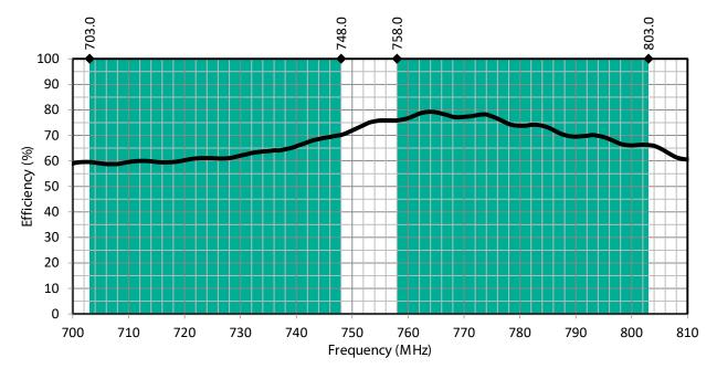
Figure 5: CW LTE Band 28 Antenna Radiation Efficiency with Band 28 Uplink/Downlink Highlights.
