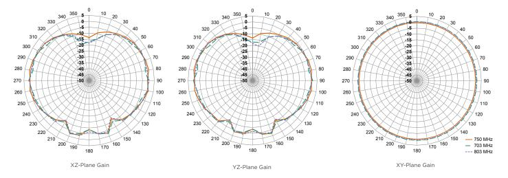
Figure 8: Radiation Patterns for CW LTE Band 28 Antenna
