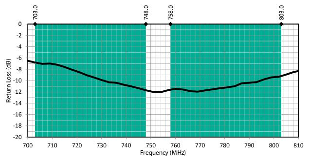
Figure 2: CW LTE Band 28 Antenna Return Loss with Band 28 Uplink/Downlink Highlights
