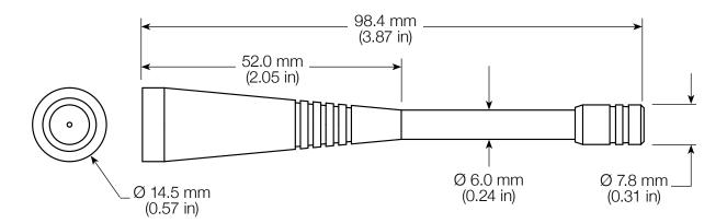
Figure 6: CW LTE Band 28 Antenna Dimensions
