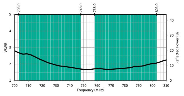
Figure 1: CW LTE Band 28 Antenna VSWR with Band 28 Uplink/Downlink Highlights
