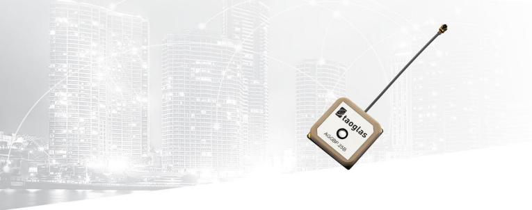
The AGGBP.25B is an internal GPS/GLONASS/GALILEO/BeiDou active patch antenna with Ø1.13 cable and IPEX MHFI connector. It is the ideal antenna for next generation GNSS devices to achieve good sensitivity across all bands in a small form factor.
