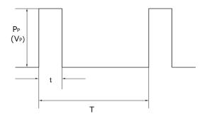
$\begin{array}{lll} P_P & : & \text{Pulse limit power (W)} \\ V_P & : & \text{Pulse limit voltage (V)} \\ t & : & \text{Pulse continuous time (s)} \end{array}$
