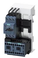
Load feeder fuseless, Reversing duty 400 V AC, Size S00 0.35...0.50 A 24 V DC screw terminal for 60 mm busbar systems (also fulfills type of coordination 1) Type of coordination 2, Iq = 150 kA 1 NC (contactor)
