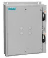
Duplex starter w/o alternator, Size 1, Three phase full voltage, Solid-state overload relay, OLR amp range 10-40A, 208VAC 60Hz coil, Combination type, Two 30A circuit breakers, Enclosure NEMA type 1, Indoor general purpose use
