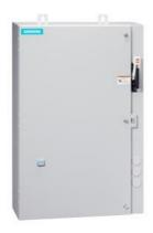
Non-reversing motor starter, Size 2 1/2, Three phase full voltage, Solidstate overload relay, OLR amp range 25-100A, 24VDC coil, Combination type, 100A non-fusible disconnect, Enclosure NEMA type 4/12, Water/dust tight for outdoors, Standard width enclosure
