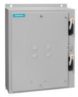
Duplex starter w/o alternator Size 2 Three phase full voltage Solid-state overload relay OLR amp range 13-52A 24VAC 50-60Hz Coil Combination type Two 60A disconnect switches Enclosure NEMA type 4/12 Water/dust tight weather proof
