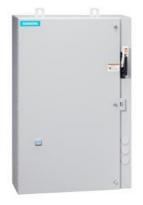
Non-reversing motor starter, Size 2, Three phase full voltage, Solid-state overload relay, OLR amp range 13-52A, 24VDC coil, Combination type, 60A fusible disconnect, 60A/250V fuse clip, Encl NEMA type 4X 304 S-Steel, Water/dust tight noncorrosive, Extra-wide enclosure
