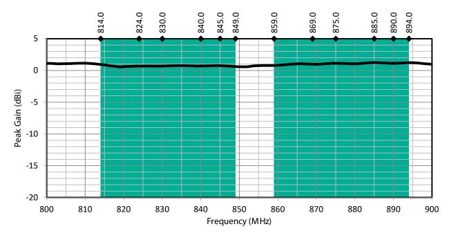
Figure 3: PW LTE Band 5 Antenna Peak Gain with Band 5 Uplink/Downlink Highlights
