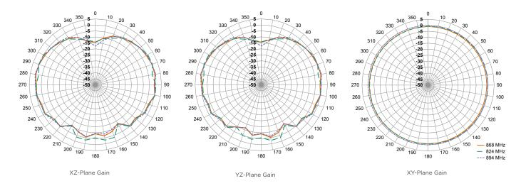
Figure 8: Radiation Patterns for PW LTE Band 5 Antenna
