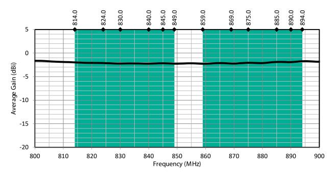
Figure 4: PW LTE Band 5 Antenna Average Gain with Band 5 Uplink/Downlink Highlights
