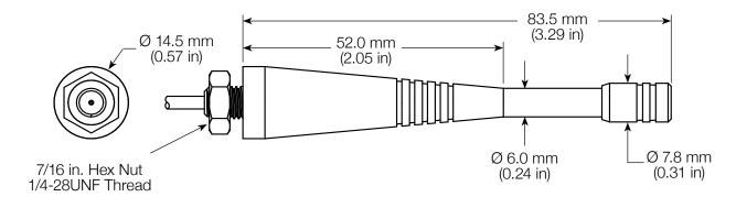
Figure 6: PW LTE Band 5 Antenna Dimensions
