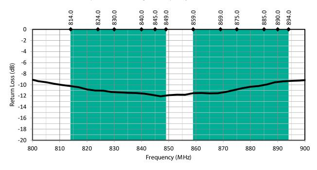
Figure 2: PW LTE Band 5 Antenna Return Loss with Band 5 Uplink/Downlink Highlights
