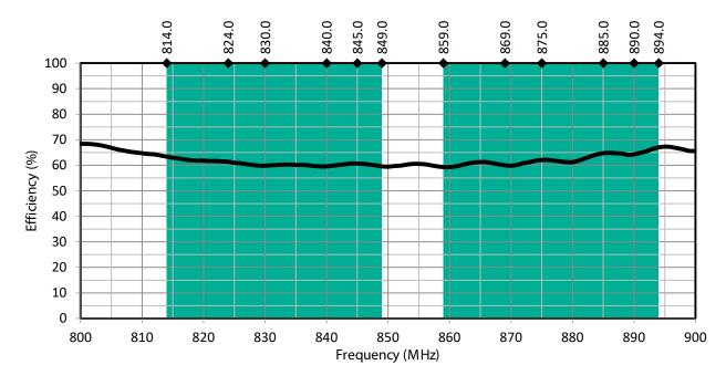
Figure 5: PW LTE Band 5 Antenna Radiation Efficiency with Band 5 Uplink/Downlink Highlights
