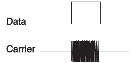
Figure 12: CPCA (AM) Modulation
