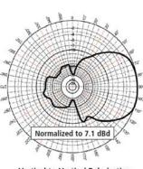
Vertical-to-Vertical Polarization Azimuthal Pattern (Y, Z, or E-plane)
