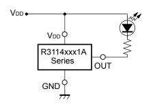
Voltage level Indicator Circuit (lighted when the power runs out) (Nch Open Drain Output)
