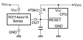
• R3114xxx1A Output Delay Time Circuit 2 (Nch Open Drain Output)
