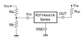
• Detector Threshold Adjustable Circuit 2 (Nch Open Drain Output)
