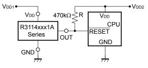
• R3114xxx1C CPU Reset Circuit (CMOS Output)
