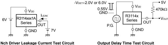
Output Delay Time Test Circuit (Pull-up circuit is not necessary for CMOS Output type.)
