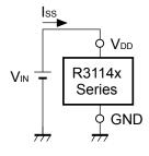
**Supply Current Test Circuit**
