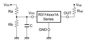
Adjustable Detector Threshold=(-VDET)×(Ra+Rb)/Rb
