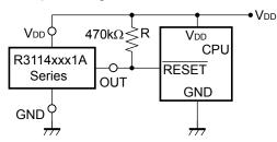
Case2. Input Voltage to R3114xxx1A is unequal to Input Voltage to CPU
