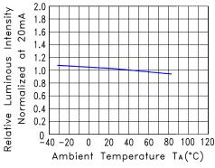
Fig.5 Relative Luminous Intensity VS. Ambient Temperature
