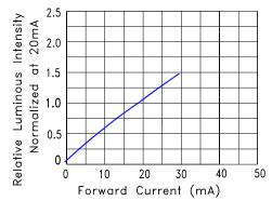
Fig.4 Relative Luminous Intensity vs. Forward Current
