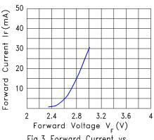
Fig.3 Forward Current vs. Forward Voltage
