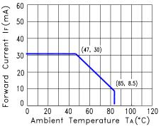
Fig.2 Forward Current Derating Curve
