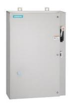
Non-reversing motor starter, Size 3, Three phase full voltage, Solid-state overload relay, OLR amp range 25-100A, 110V 50Hz / 120V 60Hz coil, Combination type, 125A circuit breaker, Encl NEMA type 4X 316 S-Steel, Water/dust tight noncorrosive, Extra-wide enclosure
