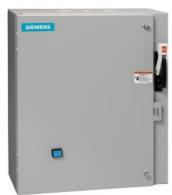
Non-reversing motor starter, Size 2, Three phase full voltage, Solid-state overload relay, OLR amp range 13-52A, 24VAC 50-60Hz coil, Combination type, 50A circuit breaker, Enclosure NEMA type 1, Indoor general purpose use, Extra-wide enclosure
