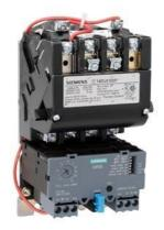
Non-reversing motor starter Size 1 Three phase full voltage Solid-state overload relay OLRelay amp range 10-40a 24VAC 50-60HZ coil Combination type No enclosure
