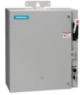
Pump control panel, Size 1 3/4, Three phase full voltage, Solid-state overload relay, OLR amp range 10-40A, 190-220/220-240V 50/60Hz coil, Standard type contactor, 40A circuit breaker, HOA Sel Sw. <(>&<)> Start P.B., Enclosure NEMA type 3/3R, Weather proof outdoor use
