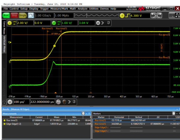
Figure 5. Power Up, 100 \mu\text{s} , V_{BIAS} = 6.5\text{ V} , R_{BIAS} = 0.5\text{ k}\Omega
