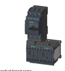
Fuseless motor starter Reversing operation 600VAC Size S00 0.22-0.32a 24V DC screw connection For screw mounting Or 35 mm rail-mounting Type of coordination 2 IQ = 150 KA Also full fills type Of coordination 1 1NO+1NC (MSP) 1NC (per contactor)
