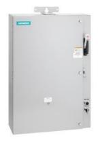
Pump control panel, Size 3 1/2, Three phase full voltage, Solid-state overload relay, OLR amp range 50-200A, 220-240/440-480VAC 60Hz coil, Standard type contactor, 200A fusible disconnect, 200A/600V fuse clip, HOA Sel Sw. <(>&<)> Start P.B., Enclosure NEMA type 3/3R, Weather proof outdoor use
