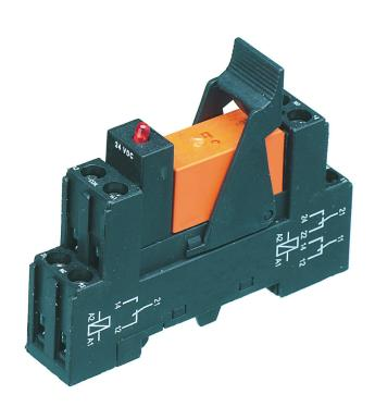
Pre-assembled relay module PRS..., Screw connection, Consisting of: relay socket base, power contact relay, pluggable display/suppression module and holding clip, 2 CO contacts, Input voltage: 110 VDC
