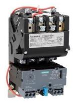
Non-reversing motor starter Size 1 3/4 Three phase full voltage Solid-state overload relay OLRelay amp range 10-40a 110-120/220-240VAC 60HZ coil Combination type No enclosure
