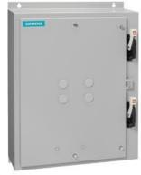
Duplex starter w/o alternator, Size 3 1/2, Three phase full voltage, Solid-state overload relay, OLR amp range 50-200A, 208VAC 60Hz coil, Combination type, Two 125A circuit breakers, Enclosure NEMA type 12, Dust/drip proof for indoors
