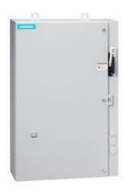
Non-reversing motor starter, Size 3, Three phase full voltage, Solid-state overload relay, OLR amp range 25-100A, 24VAC 50-60Hz coil, Combination type, 125A circuit breaker, Encl NEMA type 4X 316 S-Steel, Water/dust tight noncorrosive, Standard width enclosure
