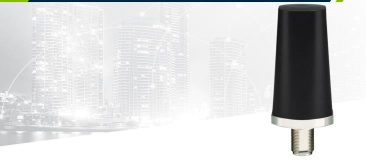
The Shockwave TLS.30.1F21 is a mechanically robust, waterproof, external antenna operating at the 433MHz band with an N type female connector. It has been designed to be used on a Ground Plane.
