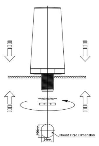
Recommended torque for mounting is 4.018 N.m or 41 kgf.cm Maximum torque for mounting is 9.8 N.m or 100 kgf.cm
